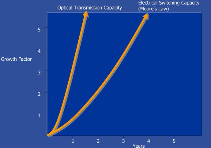
Fibre speeds overwhelming Moore's law, implying that serial OEO switching architectures have a limited future
