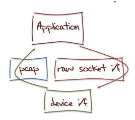
To provide a proof of concept of this approach I've been playing with such a "stateless" web server. This server responds to incoming http requests using this "stateless TCP" concept, using a "backend" conventional TCP connection to a real TCP server to generate the response (in this case the web page corresponding to the original request)
