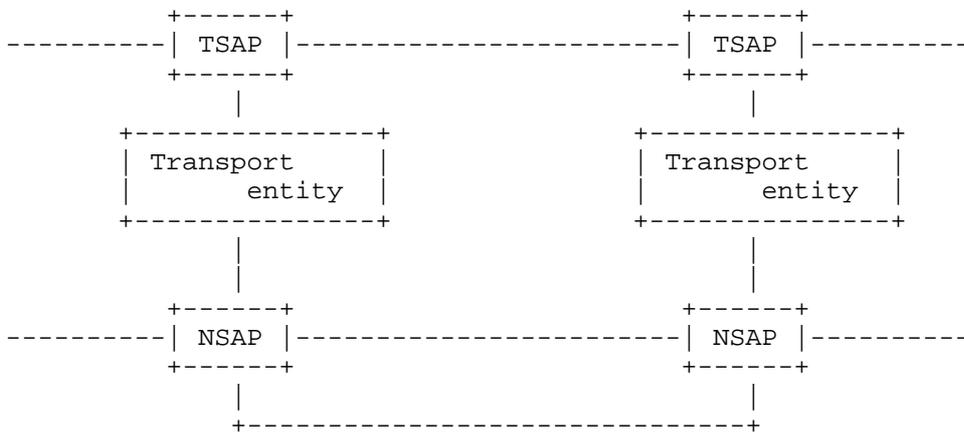
Figure 2 . Model of the transport layer
