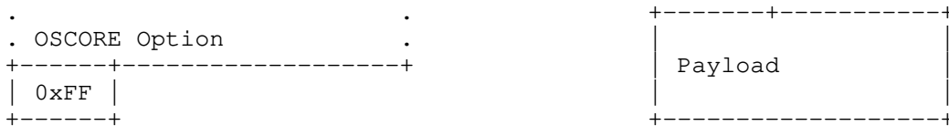
Figure 5: CoAP Packet Split into OSCORE Outer Header and Plaintext
