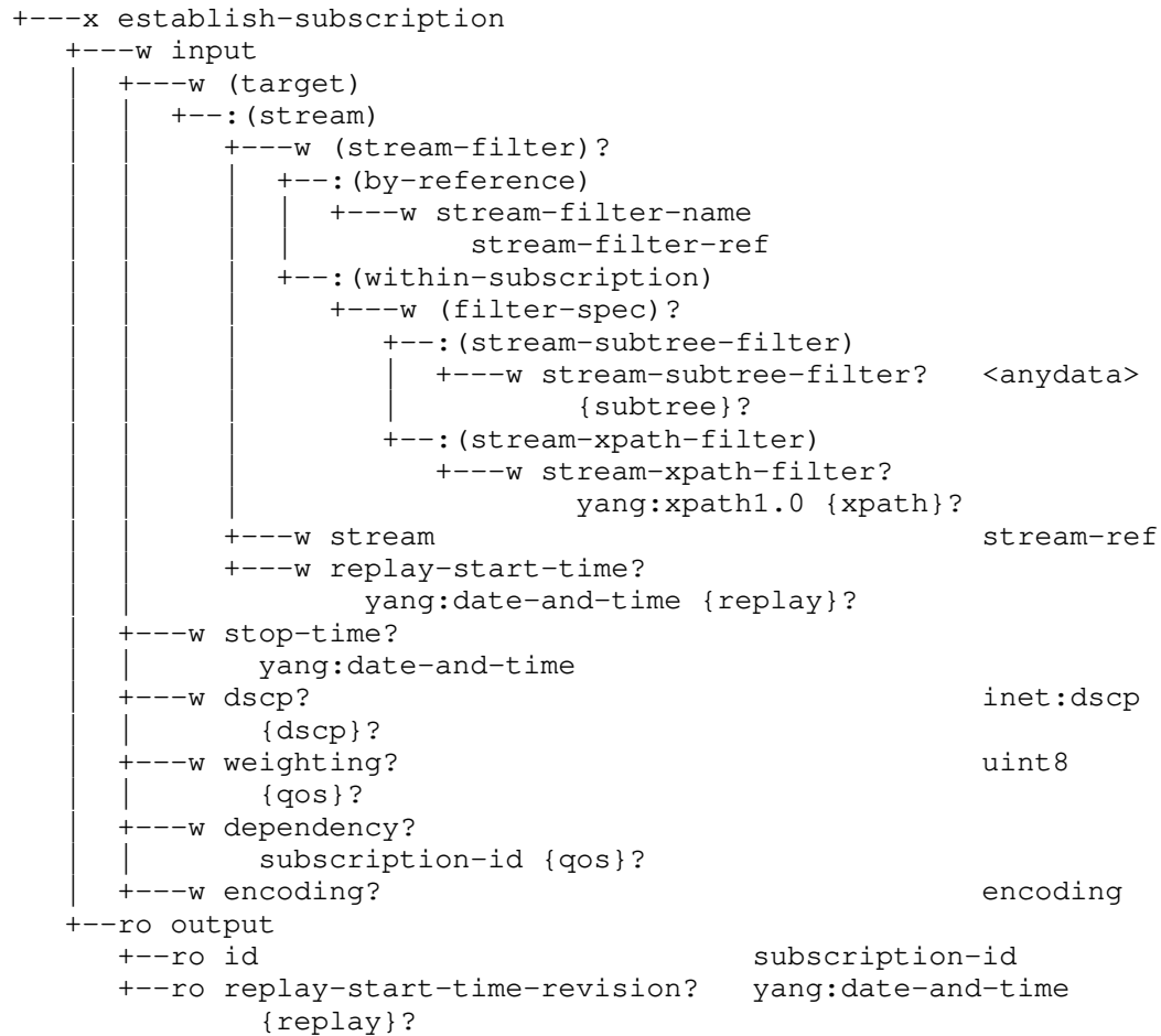
Figure 2: "establish-subscription" RPC Tree Diagram
