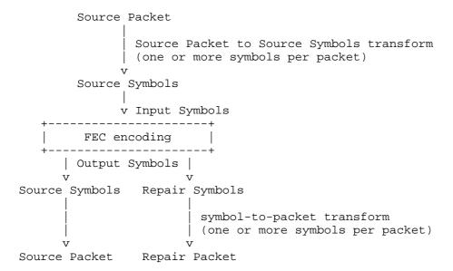
Figure 1: Packet and Symbol Relationships at a Coding Node
