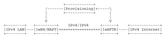
Figure 2: Lightweight 4over6 Provisioning Synchronization
