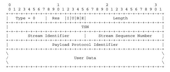
Figure 1: Extended DATA chunk format
