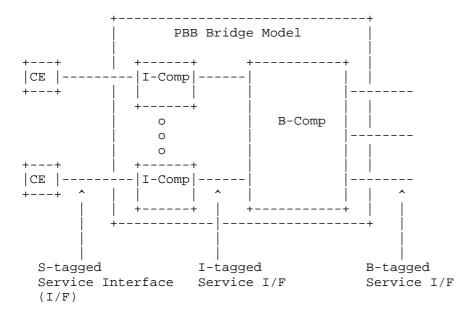
Figure 1: PBB Bridge Model
