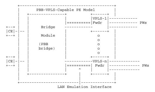
Figure 2: PBB-VPLS-Capable PE Model
