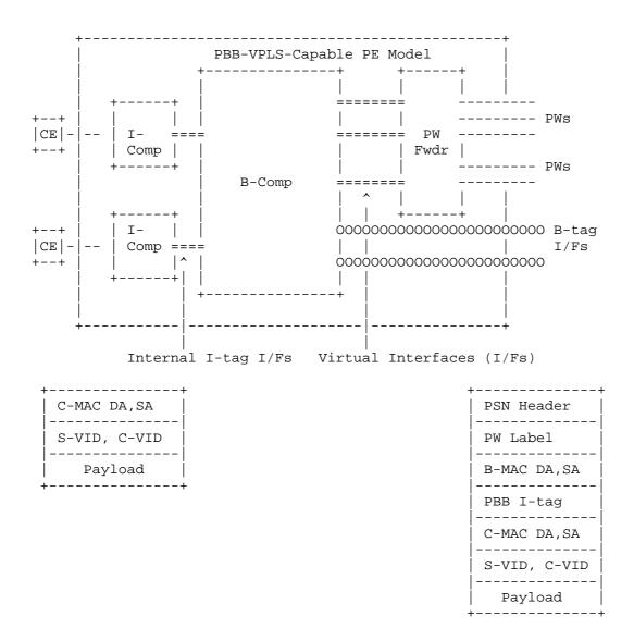
Figure 3: Packet Walkthrough for PBB VPLS PE
