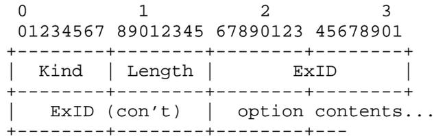
Figure 3. TCP Experimental Option with a 32-bit ExID
