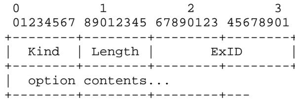
Figure 2. TCP Experimental Option with a 16-bit ExID
