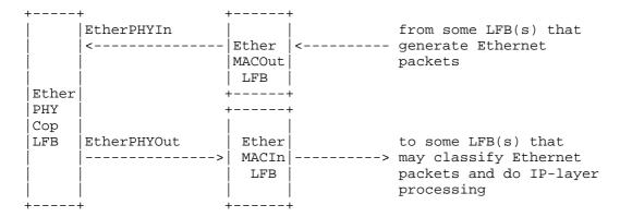
Figure 1: A Simple Sample LFB Use Case
