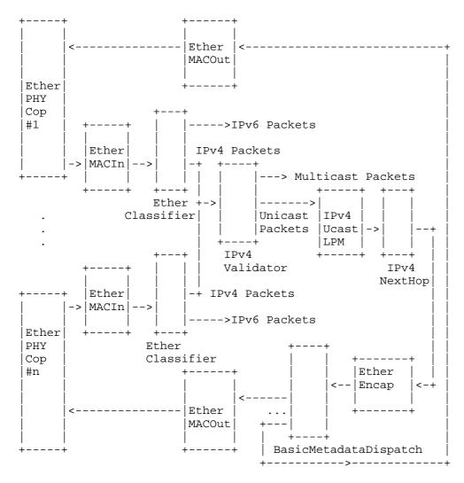
Figure 2: LFB Use Case for IPv4 Forwarding
