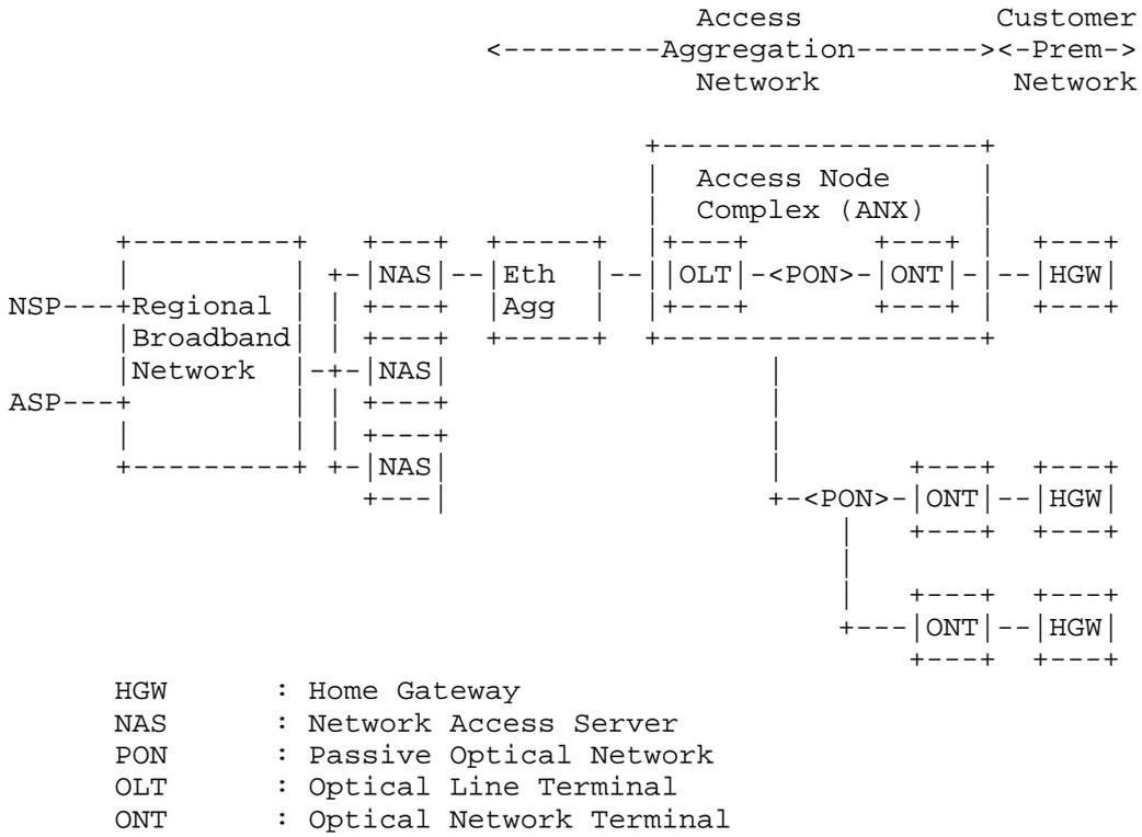
Figure 1: Access Network with PON
