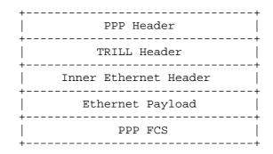
Figure 3: A PPP Encapsulated TRILL Frame
