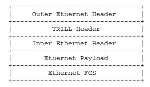
Figure 2: An Ethernet Encapsulated TRILL Frame
