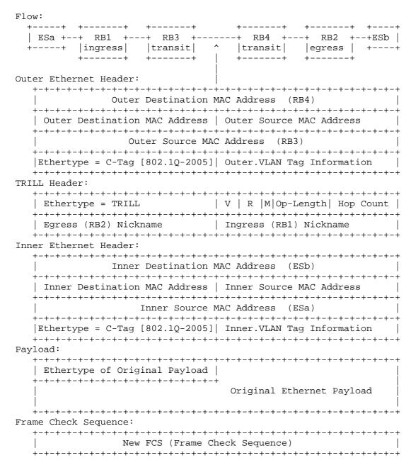
Figure 7: TRILL Data Encapsulation over Ethernet
