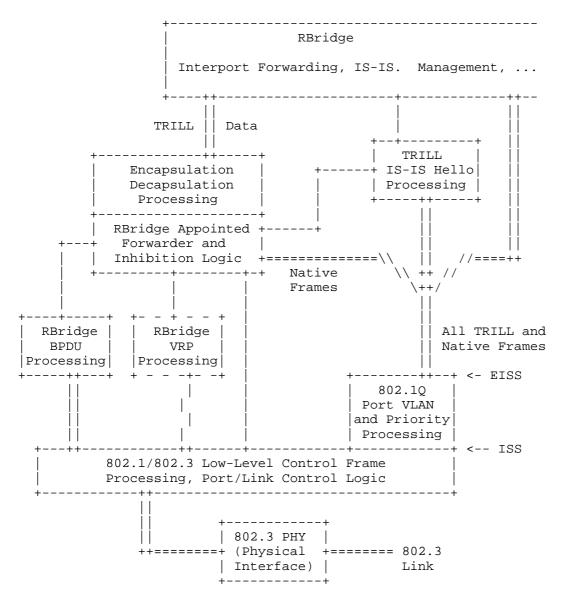
Figure 11: Detailed RBridge Port Model
