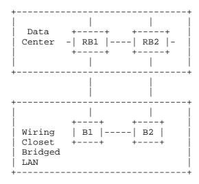
Figure 13: Wiring Closet Topology
