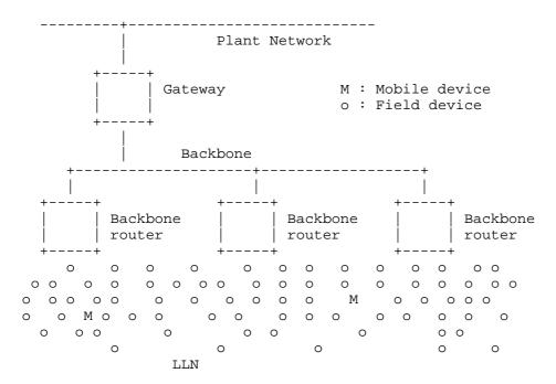
Figure 1: Backbone-Based Physical Topology
