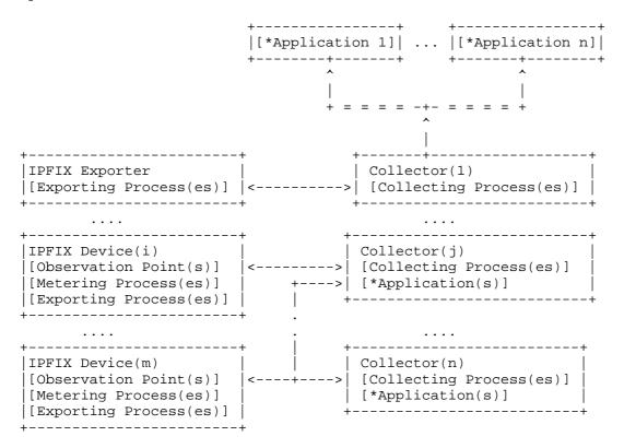
The various functional components are indicated within brackets []. The functional components within [\*] are not part of the IPFIX architecture. The interfaces shown by "<---->" are defined by the IPFIX architecture, but those shown by "<= = = =>" are not.
