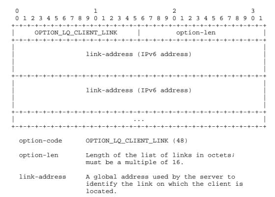
A server may respond to a query by client-id, where the 0::0 linkaddress was specified, with this option if the client is found to be on multiple links. The requestor may then repeat the query once for each link-address returned in the list, specifying the returned linkaddress. If the client is on a single link, the server SHOULD return the client's data in an OPTION\_CLIENT\_DATA option.
