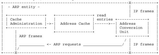
The Address Conversion Unit handles the actual conversion of IP addresses to hardware addresses. For this purpose, it uses the information in the ARP cache. The cache administration communicates with other ARP entities by ARP and creates, deletes and renews the entries in the cache.
