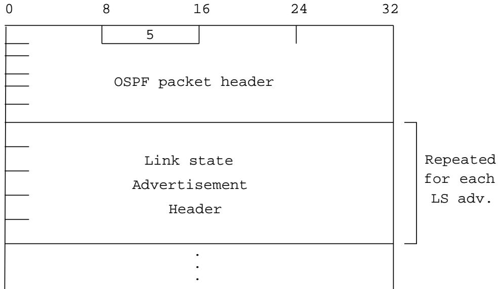
Each acknowledged link state advertisement is described by its link state header. The link state header is documented in Section A.4.1. It contains all the information required to uniquely identify both the advertisement and the advertisement's current instance.
