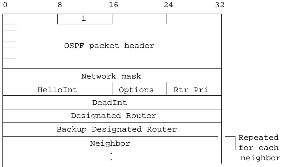
**Network mask** The network mask associated with this interface. For example, if the interface is to a class B network whose third byte is used for subnetting, the network mask is 0xffffffff00.
