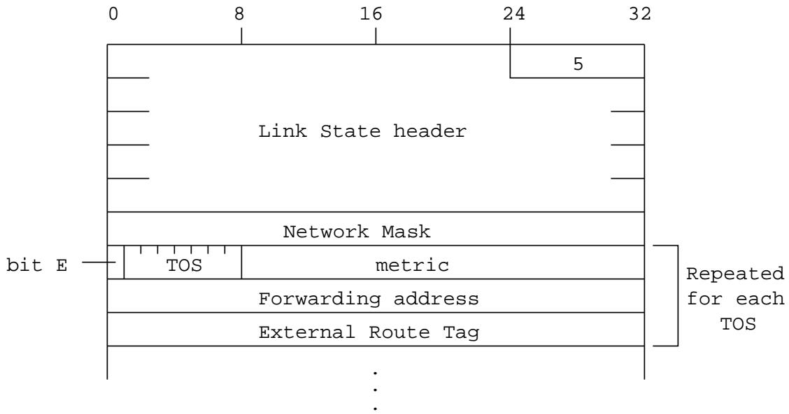
**Network Mask** The IP network mask for the advertised destination. For example, when advertising a class A network the mask 0xff000000 would be used.
