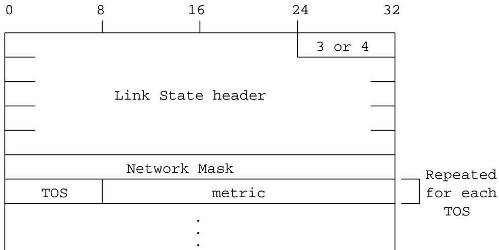
**Network Mask** For Type 3 link state advertisements, this indicates the destination's IP network mask. For example, when advertising the location of a class A network the value 0xff000000 would be used. This field is not meaningful and must be zero for Type 4 link state advertisements.
