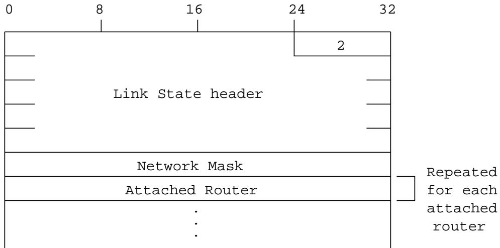
**Network Mask** The IP address mask for the network. For example, a class A network would have the mask 0xff000000.
