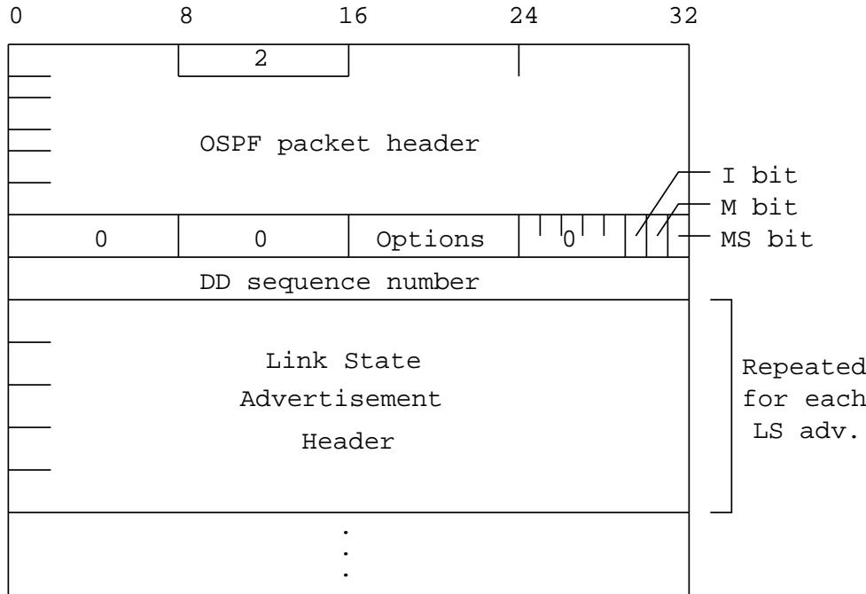
The rest of the packet consists of a (possibly partial) list of the topological database's pieces. Each link state advertisement in the database is described by its link state header. The link state header is documented in Section A.4.1. It contains all the information required to uniquely identify both the advertisement and the advertisement's current instance.
