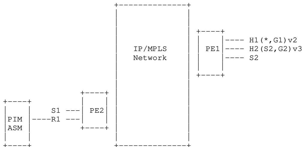
Figure 2: Multicast Router behind the EVPN Domain
