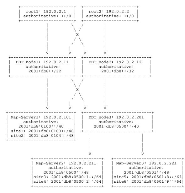
DDT nodes are configured for this "root" at IP addresses 192.0.2.1 and 192.0.2.2. DDT Map-Resolvers are configured with default referral cache entries for these addresses.
