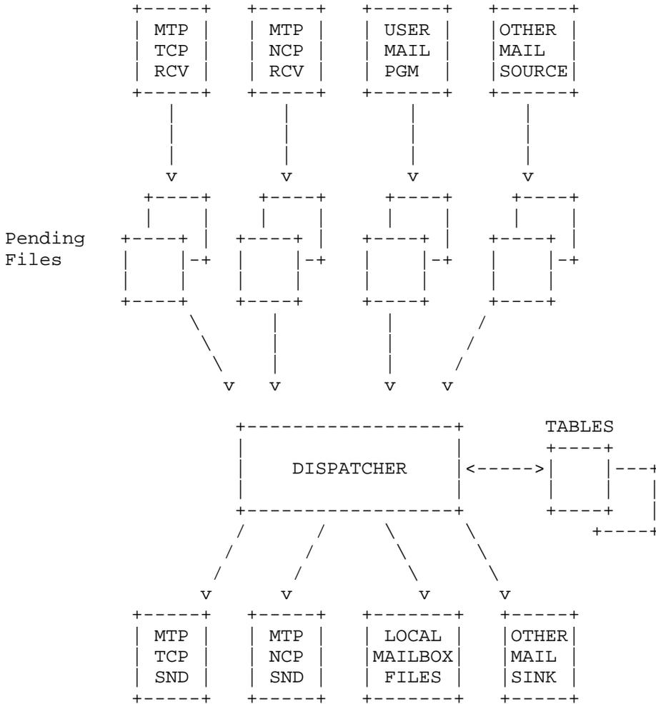
Note that current implementation the dispatcher and the senders for MTP-on-TCP and MTP-on-TCP are combined in one program.
