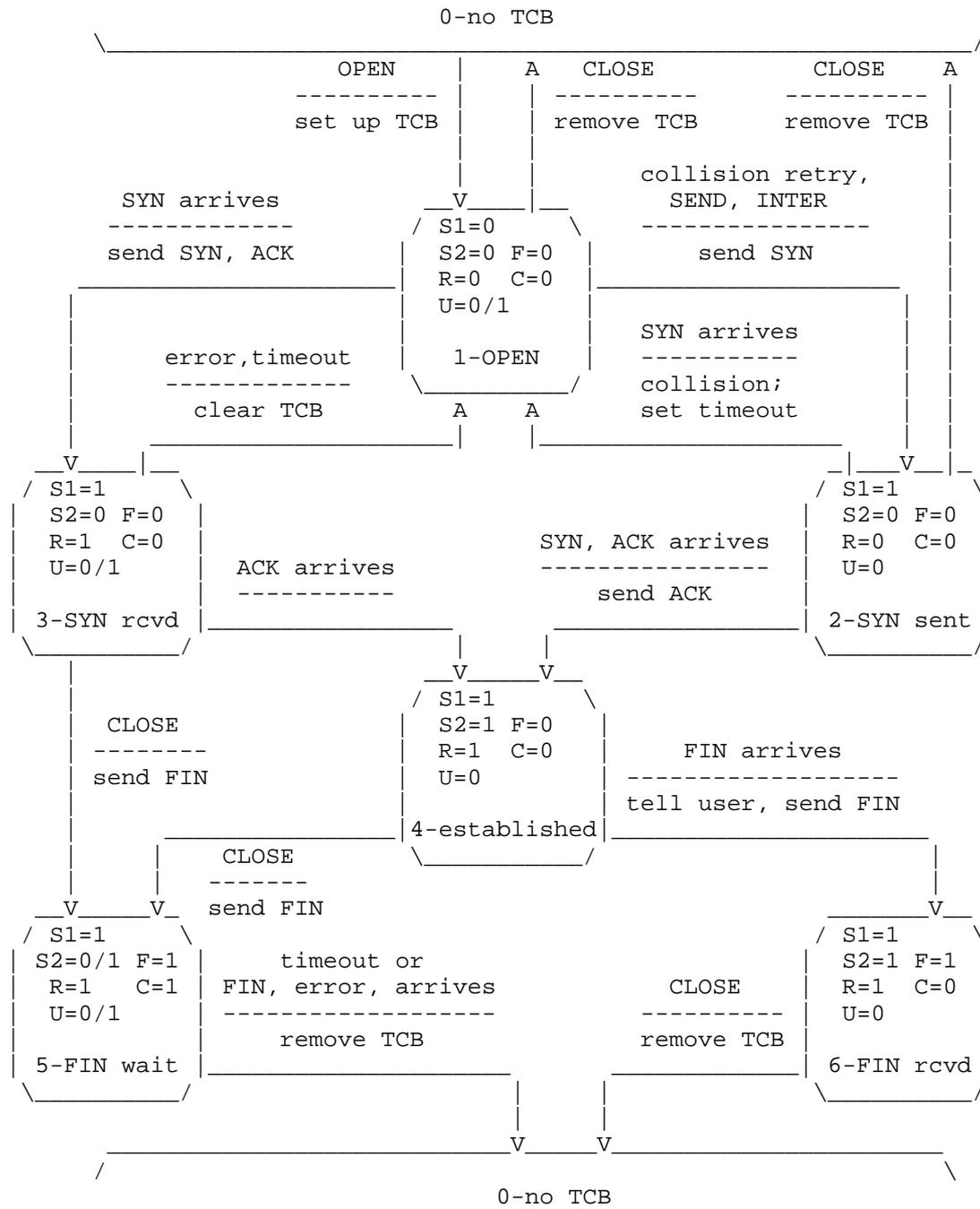
FIGURE 2.1: Structure of the TCP
