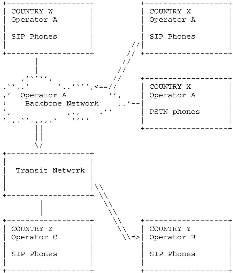
Figure 1: Example Signaling Path through Multiple Networks
