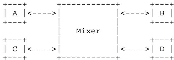
Figure 2: RTP Mixer in Unicast Only
