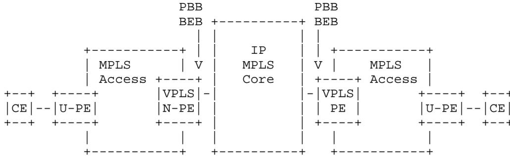
Figure 8: H-VPLS with MPLS Access Network and PBB N-PE
