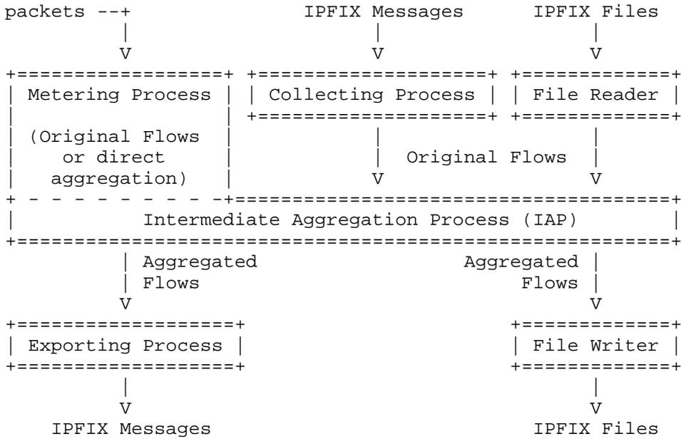
Figure 2: Data Paths through the Aggregation Process
