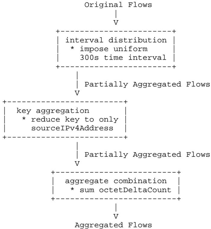
Figure 12: Aggregation Operations for Time Series per Source
