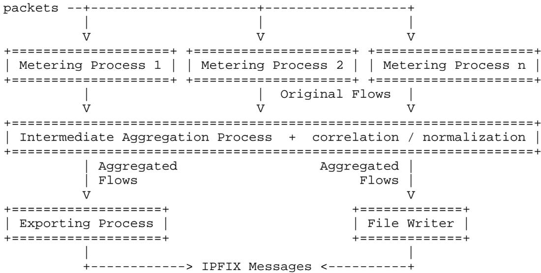
Figure 3: Aggregating Original Flows from Multiple Metering Processes
