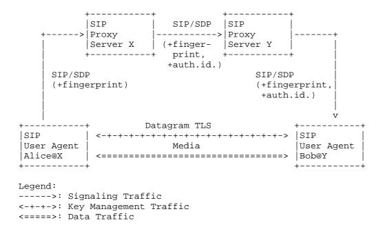
Figure 1: DTLS Usage in the SIP Trapezoid
