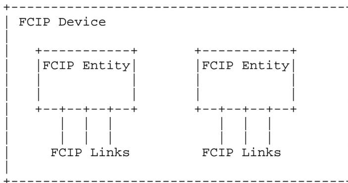
The FCIP device provides an IP-based interconnection model for interconnecting FC fabric elements. In this model, the FCIP devices along with the IP network on which they are running provide a new FCIP transport network.
