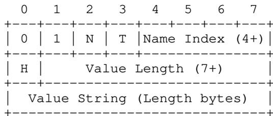
Figure 15: Literal Field Line with Name Reference
