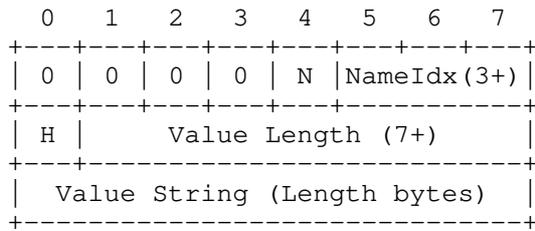
Figure 16: Literal Field Line with Post-Base Name Reference
