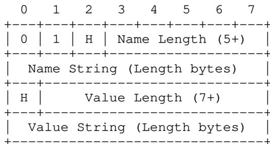
Figure 7: Insert Field Line -- New Name
