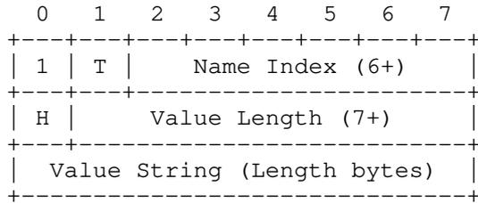
Figure 6: Insert Field Line -- Indexed Name
