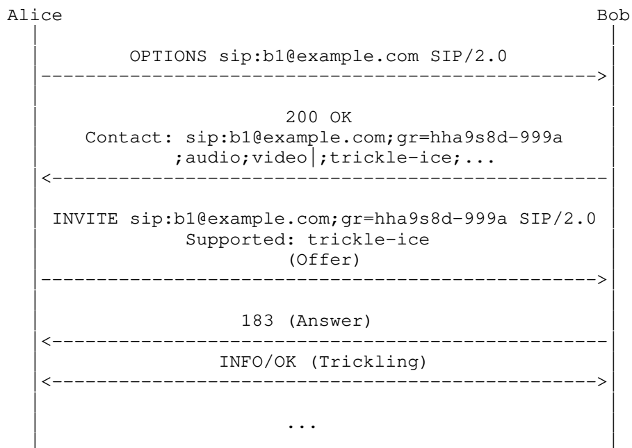
Figure 8: Trickle ICE Support Discovery with OPTIONS and GRUU
