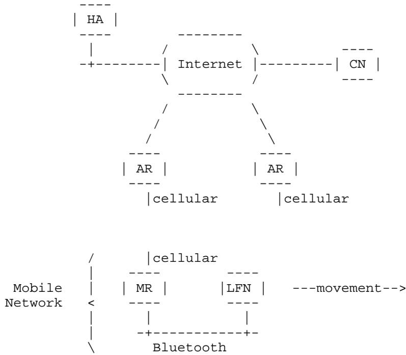
The camera (Local Fixed Node) uploads photographic content to a Correspondent Node (CN) server. When the Mobile Network moves away, the Mobile Router serving the Mobile Network changes its point of attachment from one cellular access (Access Router) to another, obtaining a new Care-of Address. The Home Agent (HA) encapsulates application traffic for the CN and LFN.
