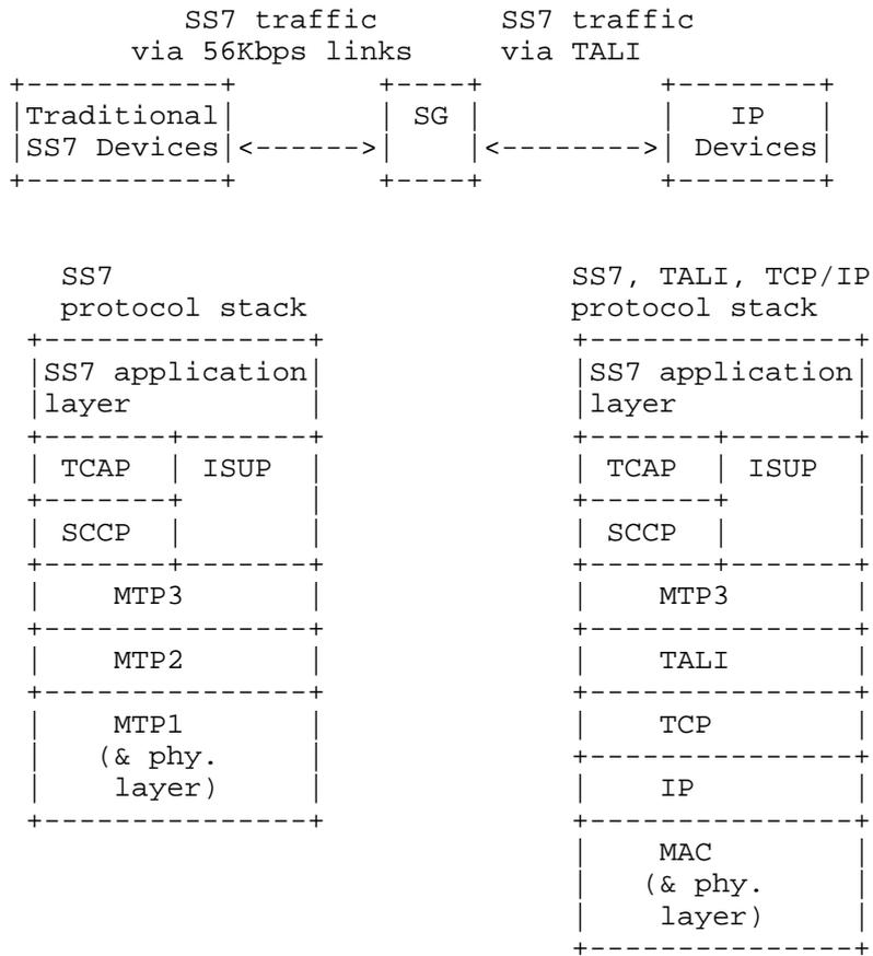
Figure 3: TALI Protocol to carry SS7 over TCP/IP
