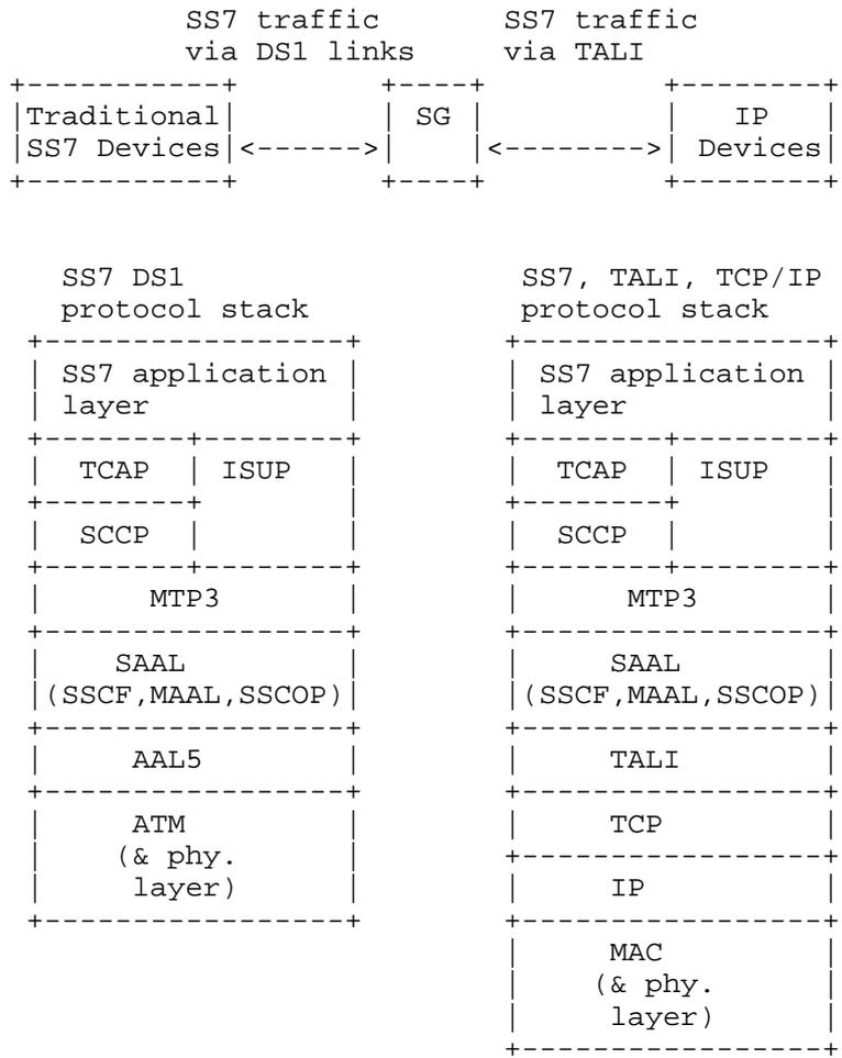
Figure 4: An Alternate TALI Protocol Stack with SAAL
