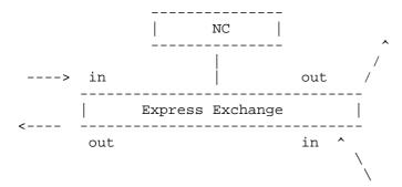
The above figure illustrates the two major functions with messages travelling in both directions and directly through the Express Exchange, except in the case of messages that must be acted on by the Net Controller. These messages will be explained in detail later.
