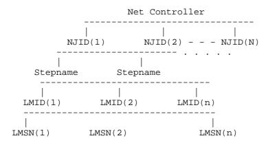
The Express Exchange is a combination of functions. It is basically a communication handler and store and forward switch. The 'EE' has the ability to keep track of all messages in the network by TEN (defined earlier). It is therefore possible to record and reflect the entire status of the network down to any detail desired.
