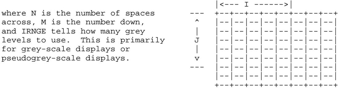
On a Gould Electrostatic Printer-Plotter, for example, the system would expect to have dot patterns with which to fill areas in order to simulate the greys. For purposes of other displays, a SETSQUARES procedure should be available so that the user can specify various kinds of cross-hatching and character filling to apply to the grid areas.
