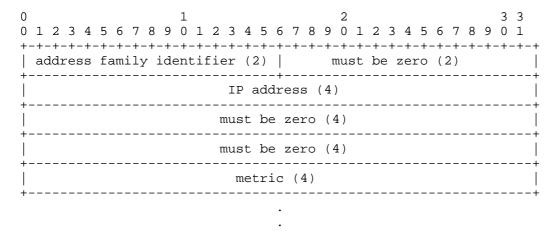
The format of an IP RIP datagram in octets, with each tick mark representing one bit. All fields are in network order.
