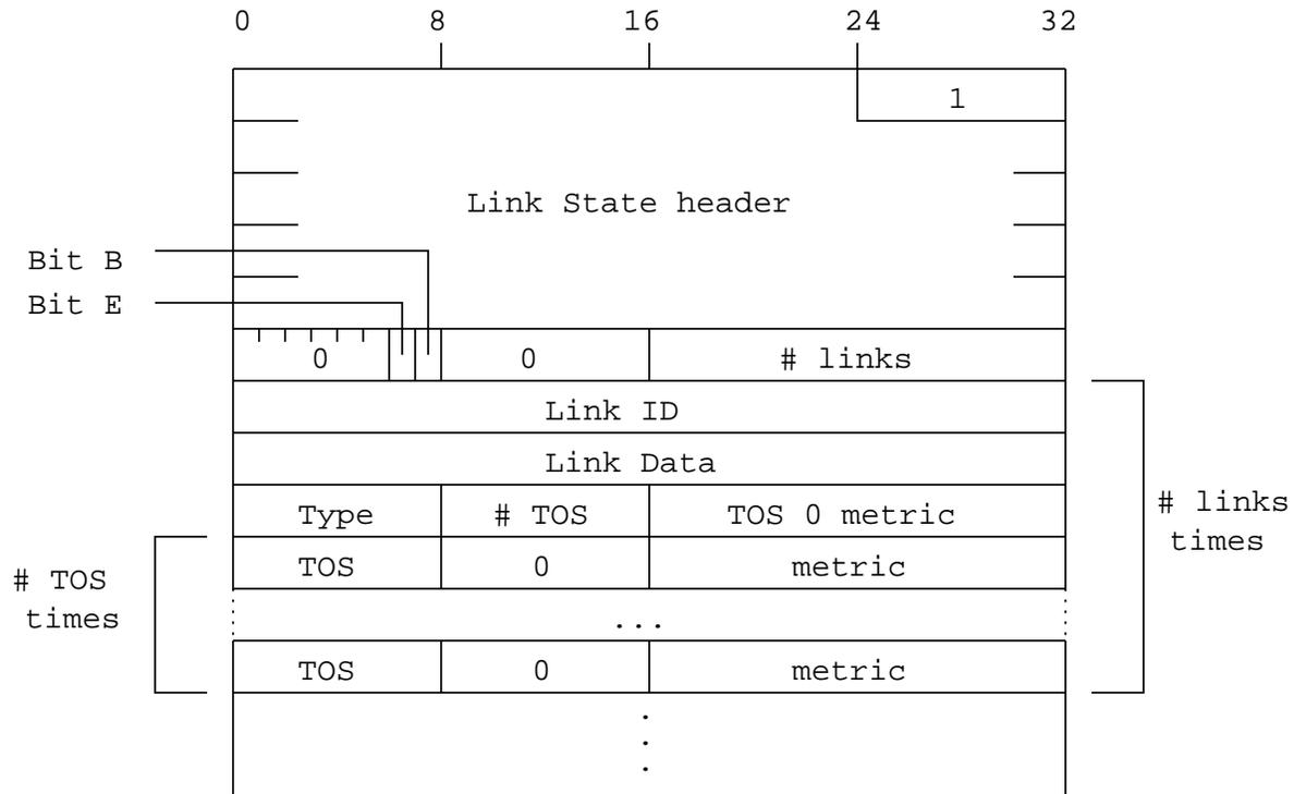
**bit E** When set, the router is an AS boundary router (E is for external)
