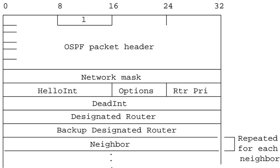
**Network mask** The network mask associated with this interface. For example, if the interface is to a class B network whose third byte is used for subnetting, the network mask is `0xfffff00`.
