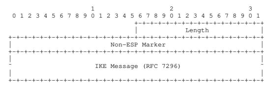
Figure 1: IKE Message Format for TCP Encapsulation
