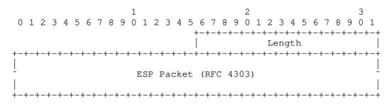
Figure 2: ESP Packet Format for TCP Encapsulation
