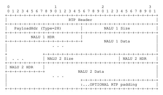
Figure 7: An Example of an AP Packet Containing Two Aggregation Units without the DONL Field
