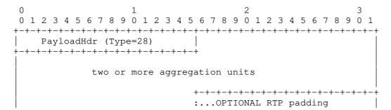
Figure 4: The Structure of an Aggregation Packet
