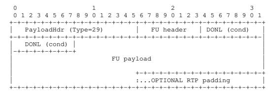
Figure 9: The Structure of an FU
