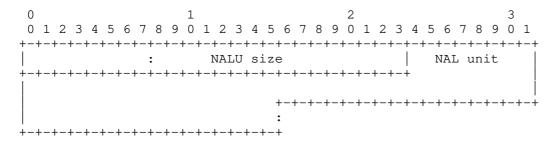
Figure 6: The Structure of an Aggregation Unit That Is Not the First Aggregation Unit in an  ${\tt AP}$
