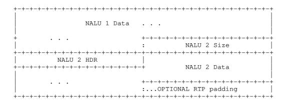
Figure 8: An Example of an AP Containing Two Aggregation Units with the DONL Field
