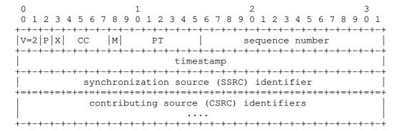
Figure 2: RTP Header According to RFC 3550
