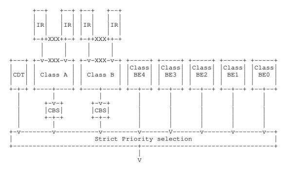
Figure 4: The Architecture of an Output Port inside a Relay Node with Interleaved Regulators (IRs) and a Credit-Based Shaper (CBS)
