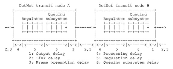
Figure 1: Timing Model for DetNet or TSN
