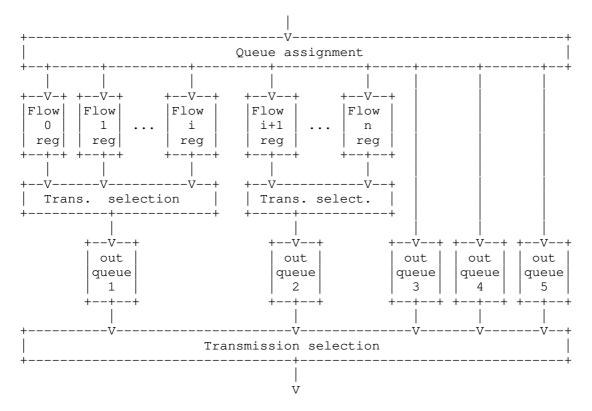
Figure 3: IEEE 802.1Q Queuing Model: Data Flow
