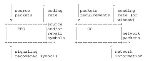
Figure 3: Separate Entities (Sender-Side)
