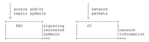
Figure 4: Separate Entities (Receiver-Side)
