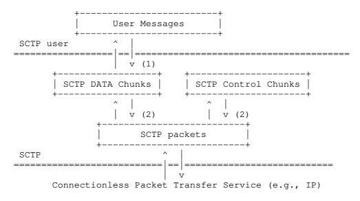
Figure 6: Illustration of User Data Transfer
