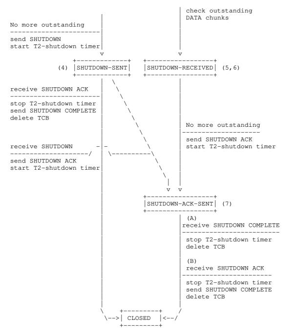
Figure 3: State Transition Diagram of SCTP
