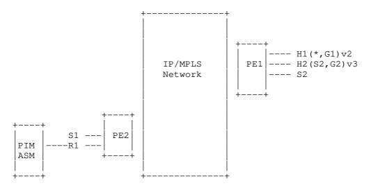
Figure 2: Multicast Router behind the EVPN Domain
