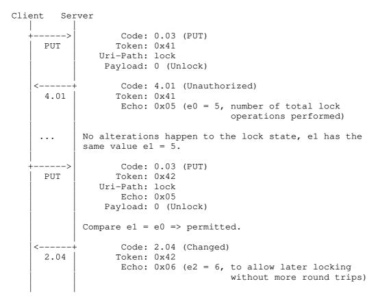
Figure 2: Example Message Flow for Event-Based Freshness Using the 'Persistent Counter' Construction of Appendix A
