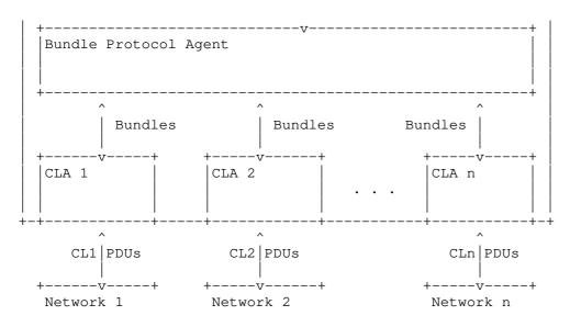
Figure 2: Components of a Bundle Node
