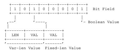
Figure 3: Compression Using a Compact Bit Field -- Bits Encode the Inclusion of TLVs
