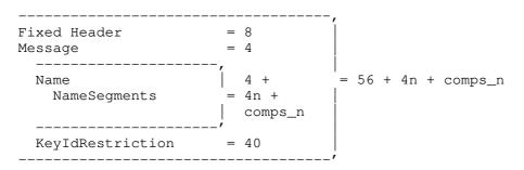
Figure 38: Estimated Size of an Uncompressed CCNx Interest Figure 39 depicts the size requirements after compression.
