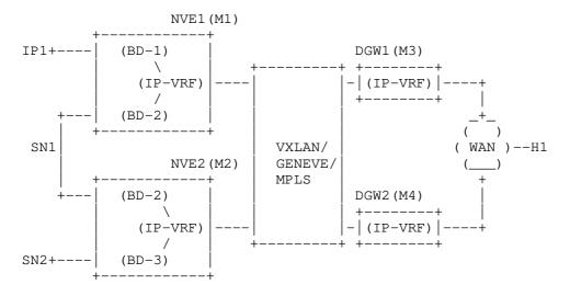
Figure 8: Interface-less IP-VRF-to-IP-VRF Model
