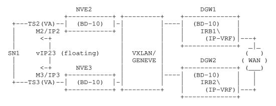
Figure 6: Floating IP Overlay Index for Redundant TS
