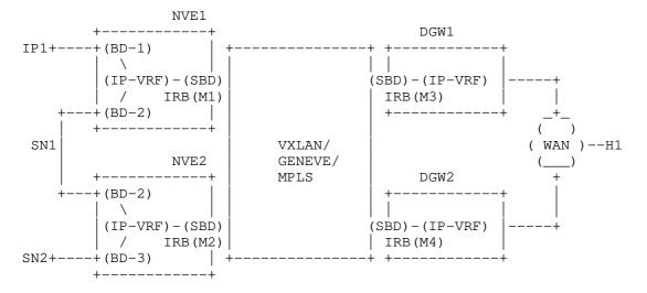
Figure 10: Interface-ful with Unnumbered SBD IRB Model
