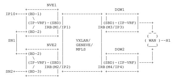
Figure 9: Interface-ful with SBD IRB Model
