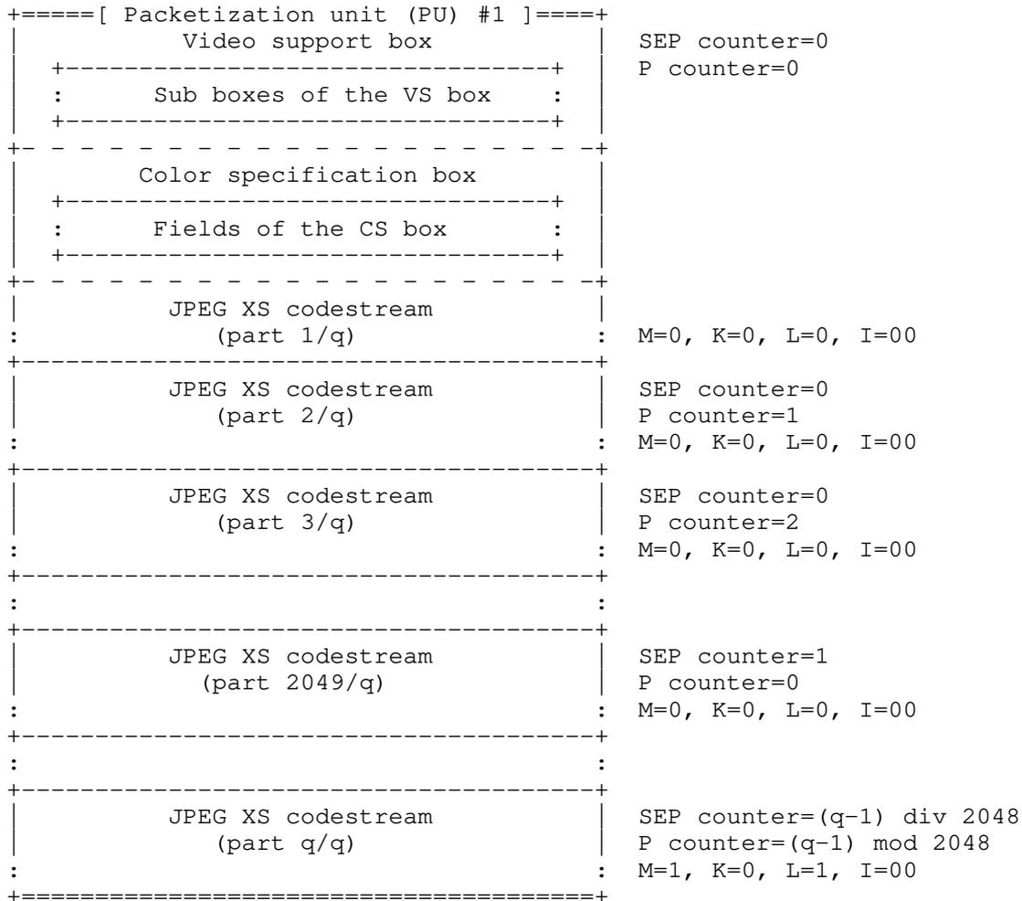
Figure 6: Example of JPEG XS Payload Data (Codestream Packetization Mode, Progressive Video Frame)
