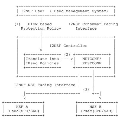
Figure 10: Host-to-Host/Gateway-to-Gateway for the IKE-less Case
