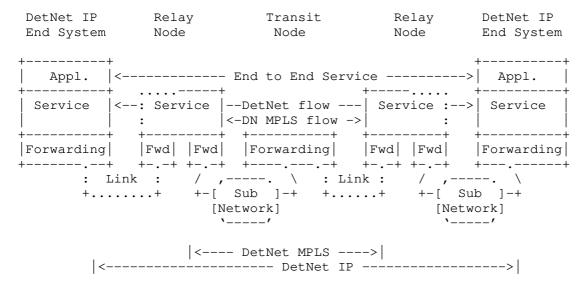
Figure 1: Architecture: DetNet IP over DetNet MPLS Network
