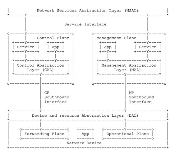
Figure 9: SDN Layers and Architecture Terminology per RFC 7426
