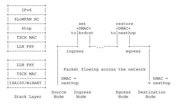
Figure 12: Track Forwarding, Tunnel Mode
