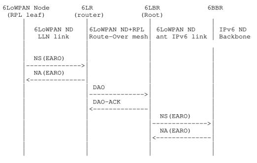
Figure 6: Next Registration Flow over Multi-Link Subnet
