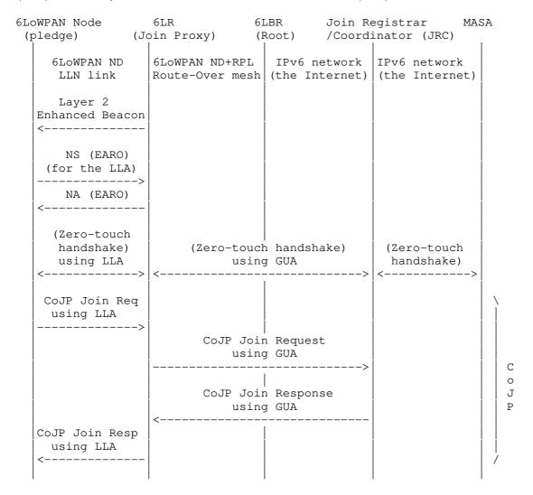
Figure 4: Join Process in a Multi-Link Subnet. Parentheses () denote optional exchanges.
