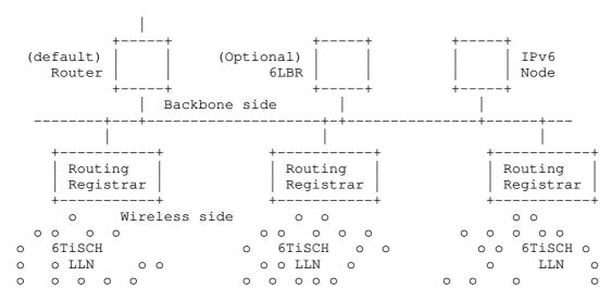
Figure 2: Extended Configuration of a 6TiSCH Network
