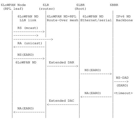
Figure 5: Initial Registration Flow over Multi-Link Subnet
