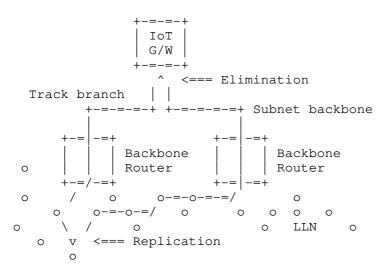
Figure 10: Example End-to-End DetNet Track
