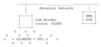
Figure 1: Basic Configuration of a 6TiSCH Network
